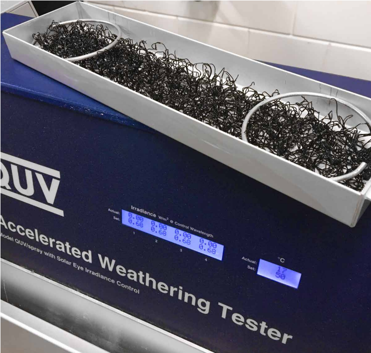
(fig. 3) Laboratory testing setup detail with EnkaMat sample
