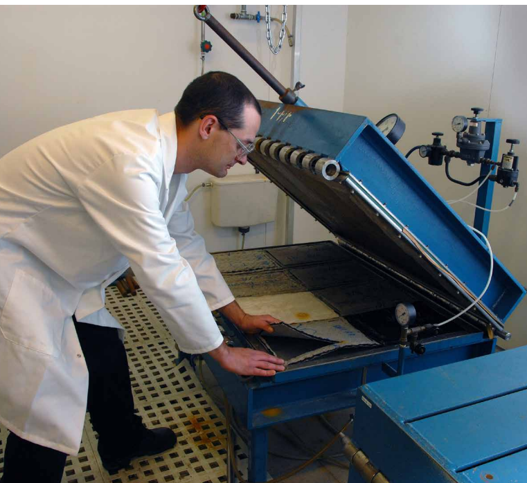
EnkaSolutions compressive creep test boxes for long term (>10 years) tests, 20-400 kPa loads.
