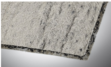
EnkaDrain® EnkaDrain 10 or 20 mm thick with drainage core consisting of looped filaments, thermobonded with one or two fleeces. 1 m wide.
