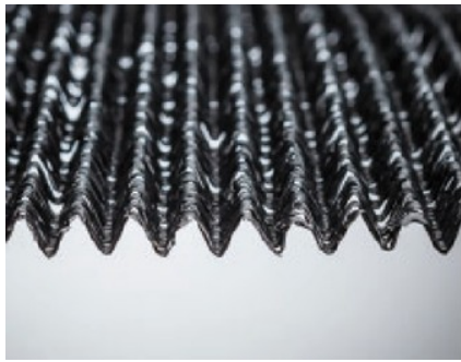
Fig. 8 – Lay rolls perpendicular to the drainage collection pipe(s). Channel direction = direction of water flow.
