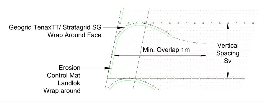
Tenax TT geogrids to be butted up against adjacent grids, or alternatively one rib to be overlapped with adjacent grids.
