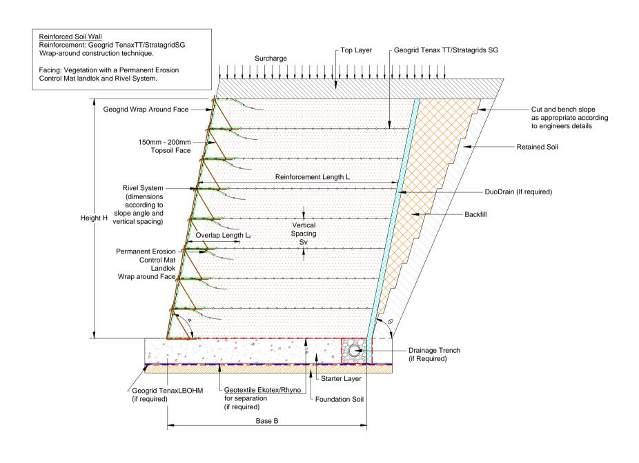
Project: Reinforced Soil Wall with Rivel System Detail
