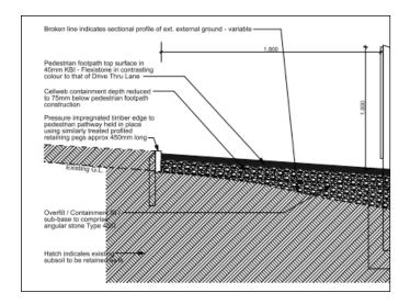
C7 Architects finalised all the designs in July 2016 and with the help of the Geosynthetics' engineers, the build-up for the drive-thru and the footpath was specified.
